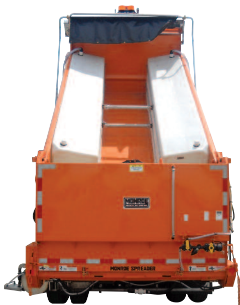
In-Bed Tank Pre-wet System
