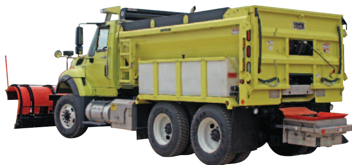
Fender Mounted Pre-wet System
