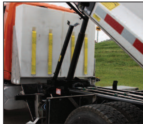
Behind the Cab Pre-wet System
